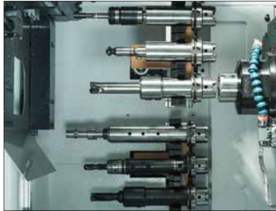
Automatic tool changer with 6 positions
