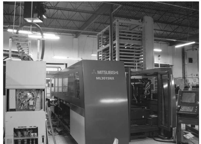
The Mitsubishi ML3015 NX laser with a 4,000 watt 40CF-R resonator and Auto-Flex MS automation, supported with a 16-shelf tower. Photo courtesy of Hansen Industries.
