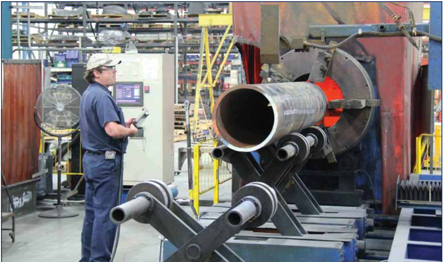
Operator sets up inch and a half thick pipe on the company’s Maruhide 6-axis plasma pipe cutting machine.
